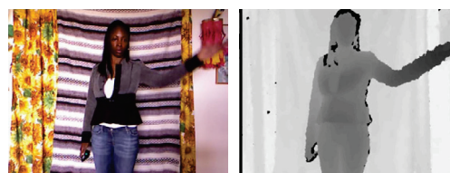
(a) RGB image (b) Depth image Fig. 1. RGB image and depth image.
